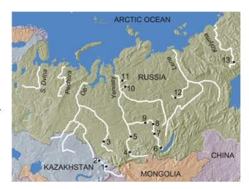
**Figure 2.** Locations of major dams (reservoir capacity >1 km<sup>3</sup>) in the watersheds of the six largest Eurasian Arctic rivers: 1, Bukhtarminskoe; 2, Shul'binskoe; 3, Novosibirskoe; 4, Sayano-Shushenskoe; 5, Krasnoyarskoe; 6, Irkutskoe; 7, Bratskoe; 8, Ust'-Ilimskoe; 9, Boguchanskoe; 10, Kureiskoe; 11, Ust'-Khantaiskoe; 12, Vilyuiskoe; and 13, Kolymskoe.
